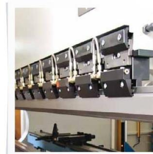
Hydraulic Tool Clamping System (O)
